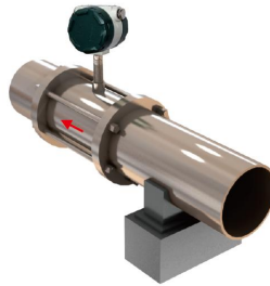
Fig.4 Schematic diagram of sensor shock absorption support
