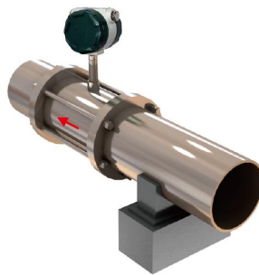
Fig.6 Schematic diagram of sensor shock absorption support
